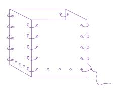
Match up the square piece with the bottom of the container. Use binder clips to hold it in place. Lace around the bottom of the container and tie it off. You're ready to put your upcycled toothbrush holder into action.
