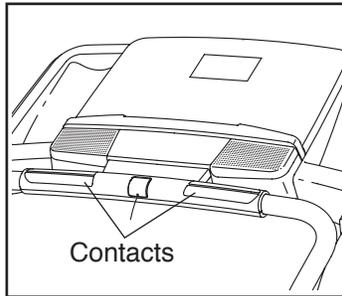
To measure your heart rate, **stand on the foot rails** and hold the pulse bar with your palms on the metal contacts for approximately ten seconds; **avoid moving your hands**. When your pulse is detected, a heart symbol in the calorie display will flash each time your heart beats, one or two dashes will appear, and then your heart rate will be shown. **For the most accurate heart rate reading, continue to hold the contacts for about 15 seconds.**
