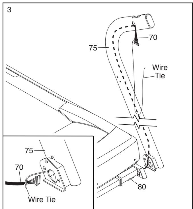
4. Hold the Left Upright (75) against the Base (80). **Be careful not to pinch the wires.** Insert a 3/8" x 3 1/2" Screw (4) with a 3/8" Star Washer (5) into the top hole in the Left Upright.
