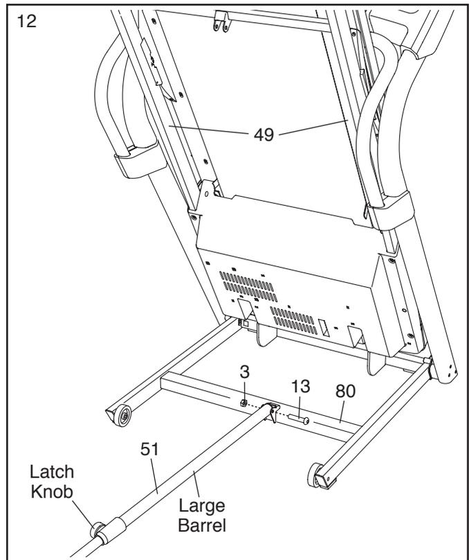
13. Attach the upper end of the Storage Latch (51) to the Frame (49) with a 3/8" x 1 3/4" Bolt (12) and a 3/8" Nut (3).
