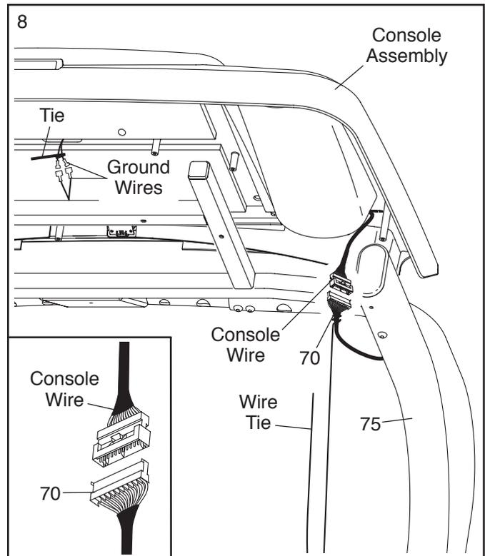
9. Insert the ground wires into the console assembly as you set the console assembly on the Left Upright (75) and the Right Upright (not shown). **Make sure that no wires are pinched.**
