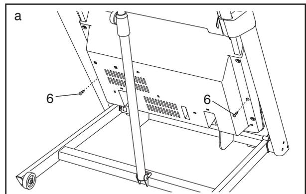
Lower the treadmill (see HOW TO LOWER THE TREADMILL FOR USE on page 22). Remove the three #8 x 3/4" Screws (6). Carefully slide the Motor Hood (57) off.
