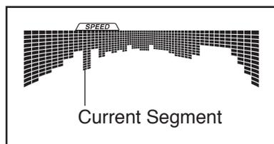
the next segment, the treadmill will automatically adjust to the new speed and/or incline setting.
