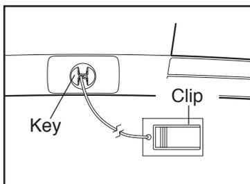
After a moment, the displays will light. **IMPORTANT:** In an emergency, the key can be pulled from the console, causing the walking belt to slow to a stop. Test the clip by carefully taking a few steps backward; if the key is not pulled from the console, adjust the position of the clip.
