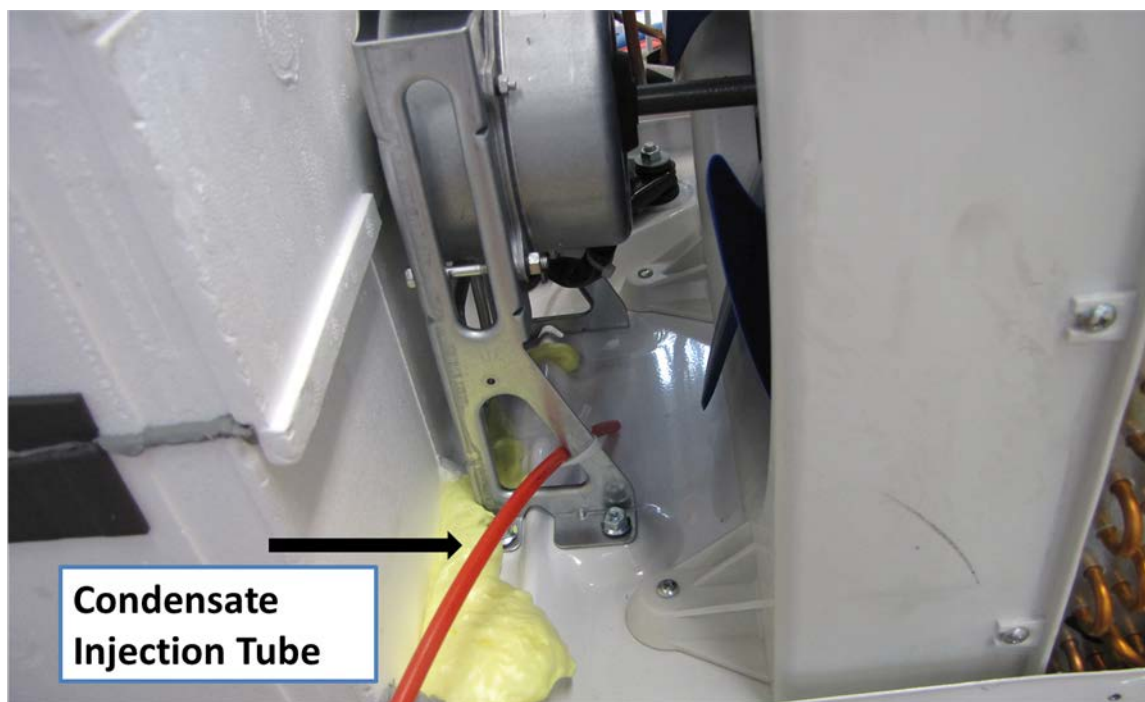
Figure 17. Condensate injection tube location just downstream of evaporator drain
