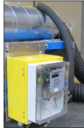
Figure 10. LFE (left), used to measure airflow rate, and chilled mirror hygrometer (right) for DP measurements
