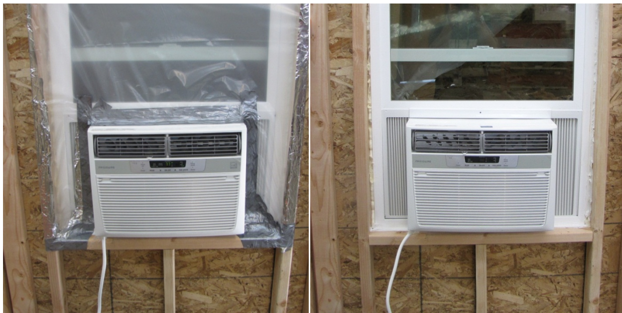
Figure 4. Example test configuration. Left: All leakage eliminated except through the unit. Right: Using only factory-supplied materials for sealing per manufacturer instructions.
