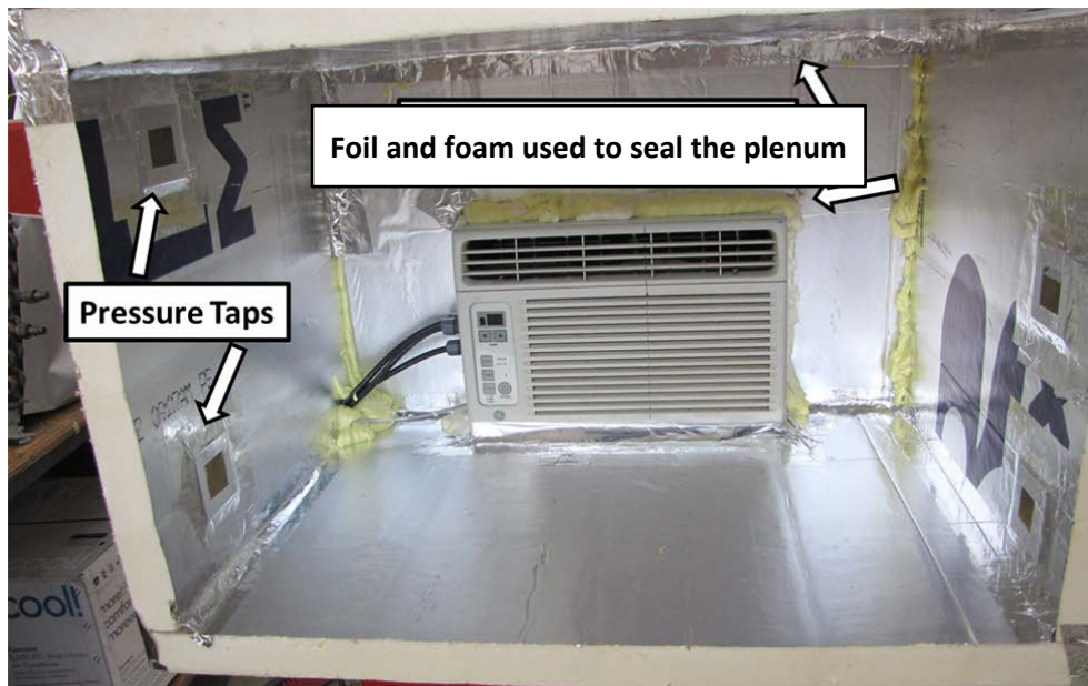
Figure 12. Front of the test unit sealed in plenum with foil tape and expanding foam
