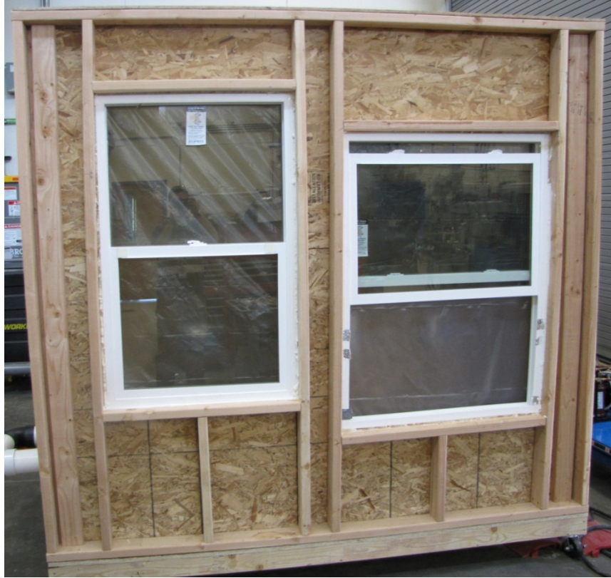
Figure 2. Test chamber used to determine air leakage around and through each window AC
