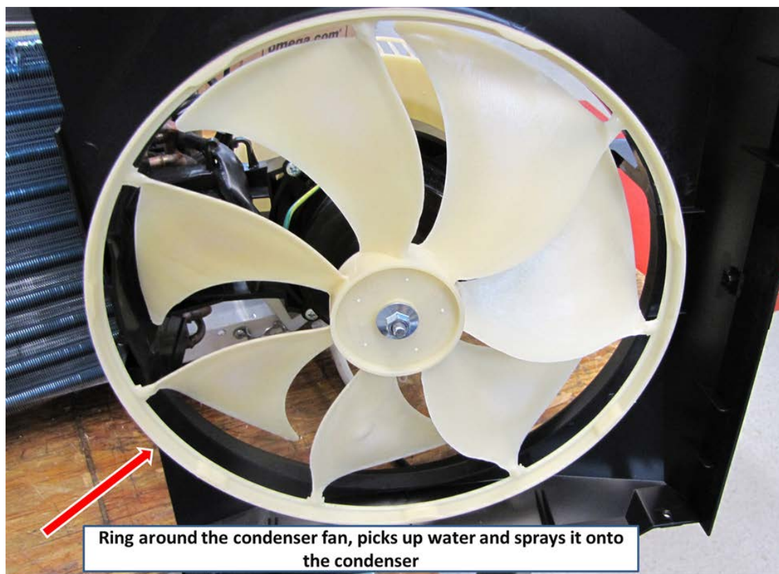
Figure 15. The condensate pick-up ring around the condenser fan
