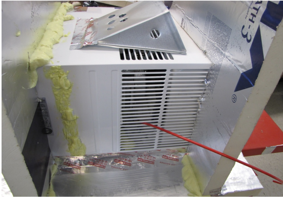
Figure 11. The center section of the plenum construction, along with the air deflector for the outdoor air return
