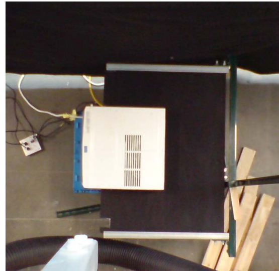
Figure 7. IR imaging test apparatus for imaging from the side (left) and from above (right)
