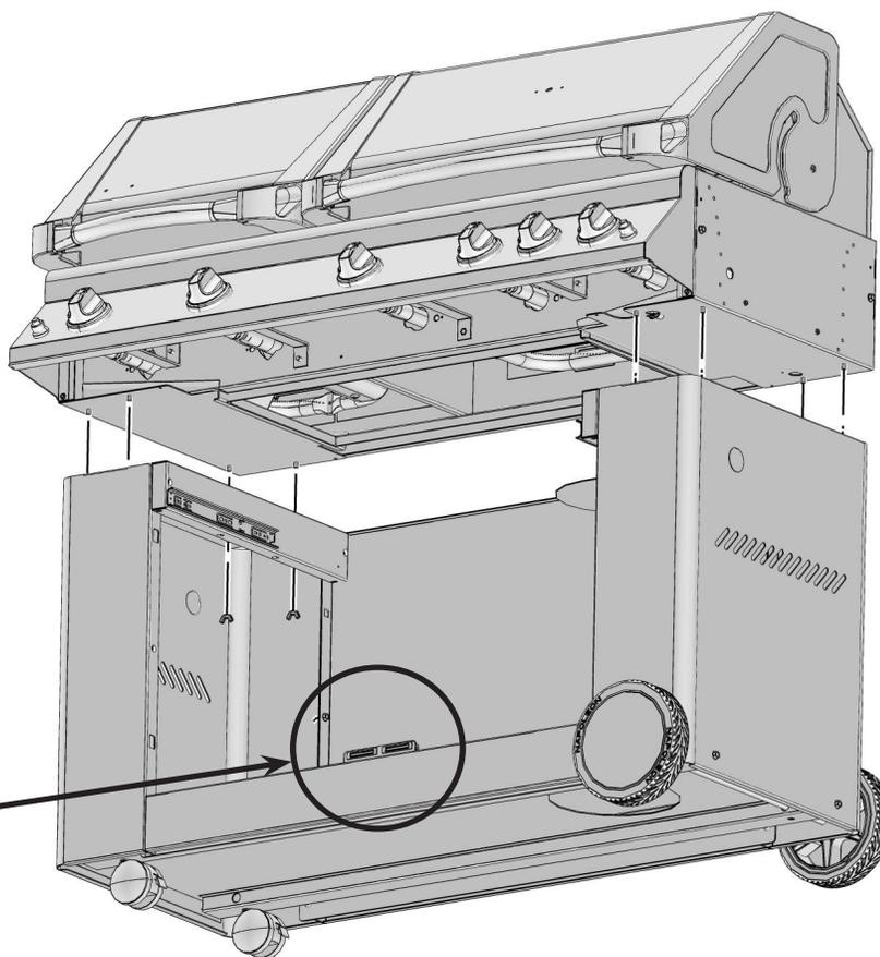
**WARNING!** Propane Only - To avoid assembly difficulties, prior to mounting the grill head, remove zip tie holding regulator. This was installed at the factory to protect the regulator hose during shipping and is no longer required. (Take care when removing the tie not to damage the hose). Ensure the regulator hose does not become pinched between the grill head and the cart.
