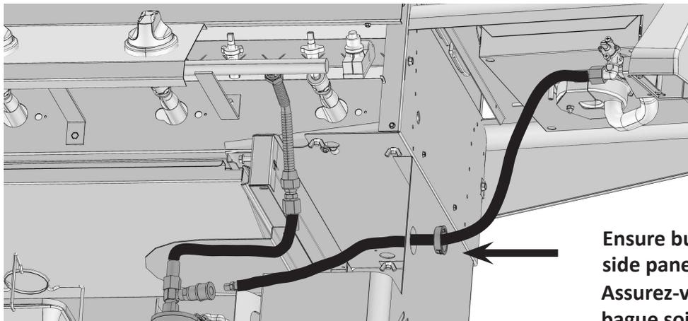
Ensure bushing snaps into side panel as shown.
