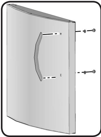
The depth of the door leveling screw will adjust the fit of the doors.
