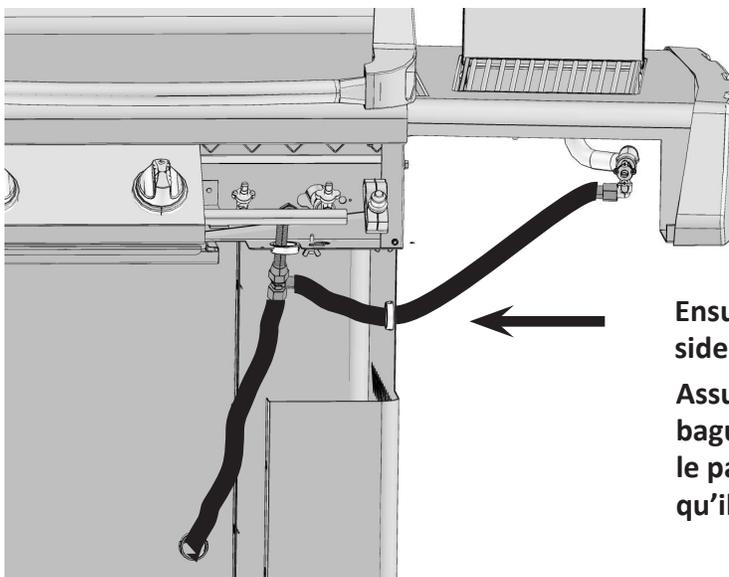
Ensure bushing snaps into side panel as shown.
