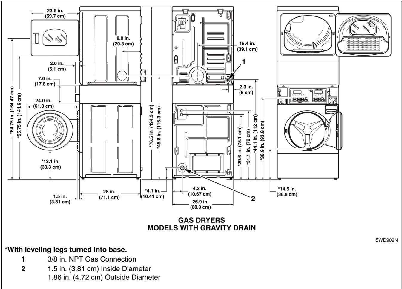
**NOTE:** Side and rear exhaust openings are 4 inch (10.2 cm) ducting. Gas models cannot be vented out left side of cabinet because of burner housing.
