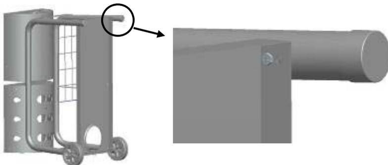
Turn grill assembly up on end as shown and tighten ALL nuts and bolts.
