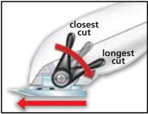
The taper lever adds versatility to your clipper by allowing you to gradually change the closeness of your cut. (Up position = closest cut; Down position = longest cut) Should the blades become jammed with hair, move the taper lever up and down several times. This will help free up the blades.
