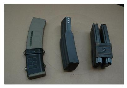
Here are 3 choices for higher capacity magazines that work. Left is a Pmag with and extension, Center is a Surefire 60 round mag and the right one is 2 military mags clamped together
