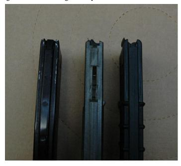
Here are three magazines to stay away from. Right is a cheap metal magazines with bent feed lips. Center is the Ramline universal with weak feed lips and the left one is a Thermold with a broken Feed lip.
