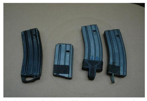
The left mag is equipped with a ranger floor plate that worked well The 20 round mag has grip tape applied to improve the grip on the slick aluminum. I always carry at least 1, 20 round magazine in case I need to get into a lower prone position.
