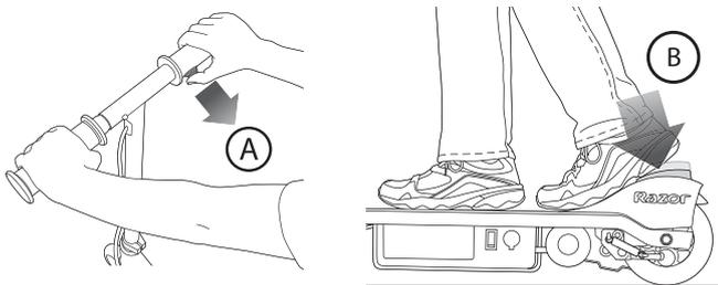
To stop unit, release the push button throttle (A) and step down on the rear fender brake (B) until the unit comes to a complete stop.
