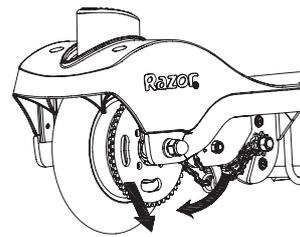
**3** To loosen the chain, push the chain tensioner down to create some slack in the chain.
