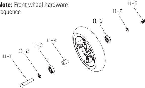
**1** Using two (2) 5mm Allen wrenches, loosen the axle bolt. Remove wheel and install replacement wheel. (Note the sequence of the hardware)
