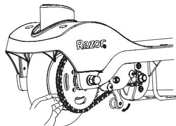
**5** Push the chain tensioner down to install the chain on both sprockets.
