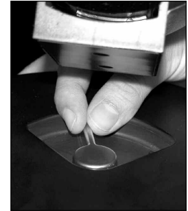
Fig. 17: Tighten horizontal lock.
