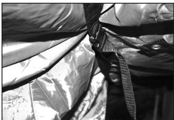
STEP 22 - Snap web strap buckles together and pull strap to tighten around SUV.
