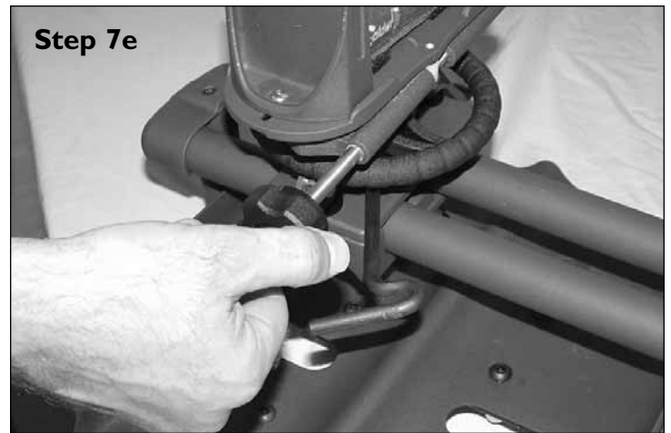
e. Spin the windage adjustment knob onto the windage adjustment shaft as shown and hand-tighten.
