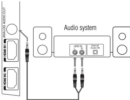
*(Sample Illustration) Connecting an analog audio system*
