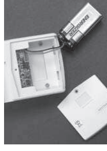
Insert 9V alkaline battery to the sensor
