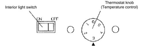
The temperature control and the interior light switch are both located on the back of the cabinet.
