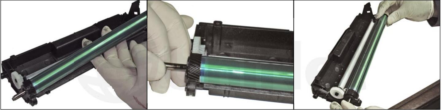
13. Clean the OPC surface and proceed to install it in the cartridge, moving the shaft inside just enough to seat the OPC drum properly. Cover the drum section away from light and set aside. Begin work on the developer section.
