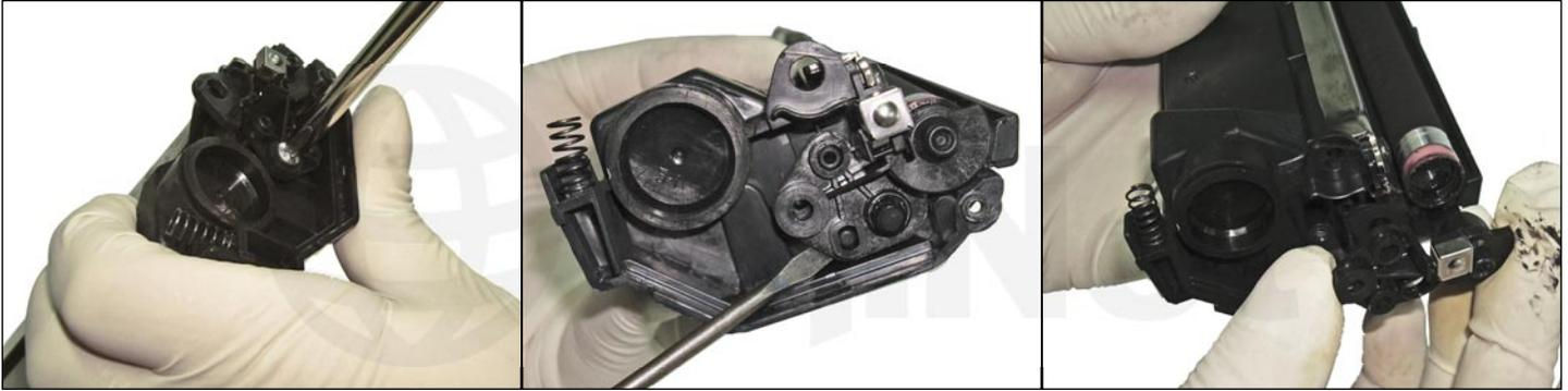
15. At the opposite end, remove the screw holding the contact end plate. It must be noted that there is NO conductive spring or blade doing the electrical work. Instead, a conductive plastic tip at the plate can be found. This is further confirmed by the use of fair amount of conductive grease both at this bearing and the inside of the metal developer roller.
