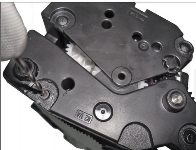
2. Mark the center of each cut and drill a hole with the small drill bit no deeper that 3/16".
