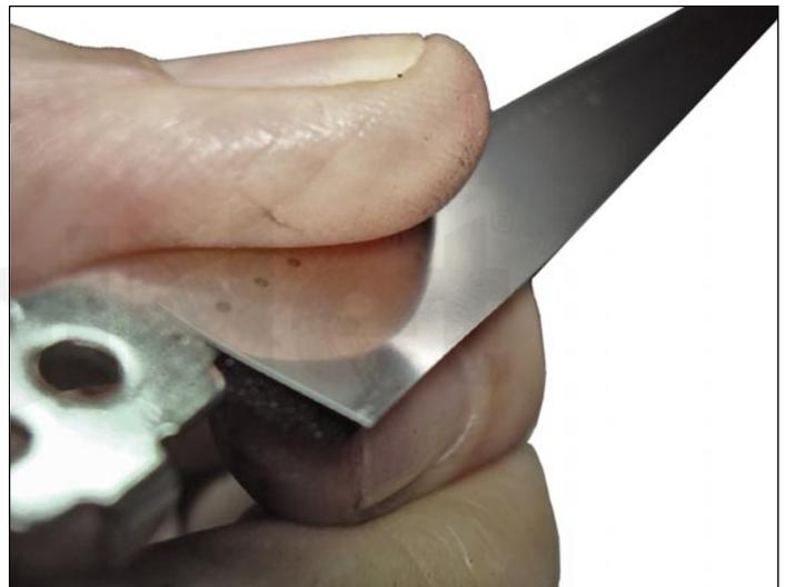
18. Remove the two Phillips screws and doctor blade from its place, then clean with a soft cloth.
