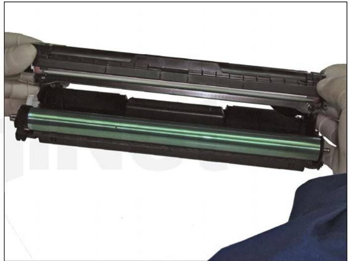
24. Now take the image section and place it on top of the developer section as shown, positioning the compression springs properly.
