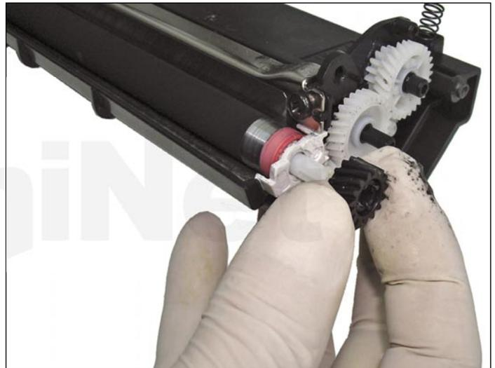
14. Remove the black gear from the developer roller, using the small screwdriver as leverage.
