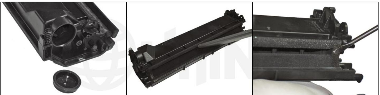
19. Vacuum the hopper completely, including the feed roller, and remove the fill plug to facilitate the work.
