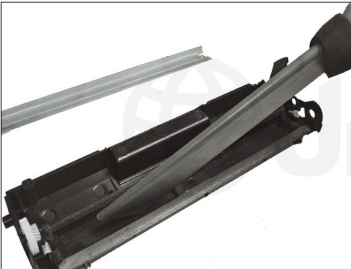
10. Vacuum the waste bin and surrounding areas. Inspect also the state of the wiper and the recovery blade seals.
