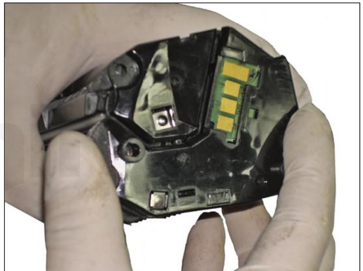
26. Work on the opposite end by taking the end cover and lubricating all contact points, and replacing the chip as shown.
