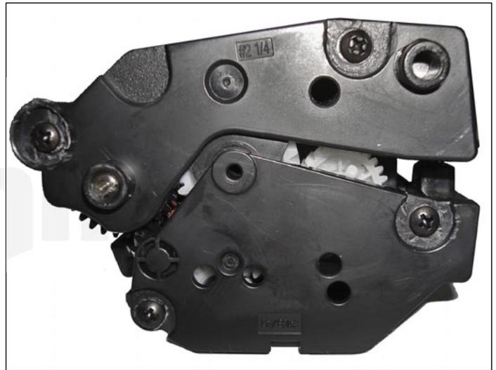
25. While holding both sections together, place the lower part of the end cover in place, matching the chamfered shaft of the OPC with the right hole. Screw the cover in place and proceed to install to larger cover in place.
