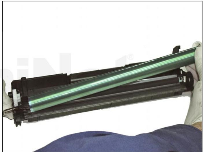
7. Slide the OPC drum axle out just enough to allow the opposite end of the drum to be lifted out of position and remove it.
