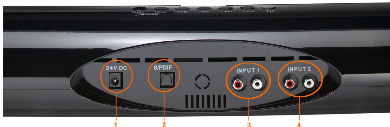
Figure 1 - Power and Input connections - HD Sound Bar System
