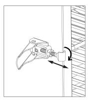
Loosen hex nut on door latch. Turn hook clockwise to tighten as shown.
