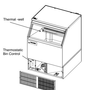
approximately 1 minute. Remove the ice. The machine should restart in approximately 3 minutes. If a major adjustment is required, turn the adjustment screw counterclockwise (warmer) until it stops then turn the adjustment screw clockwise (colder) 1/8 of a turn. This should put the control close to the proper adjustment, recheck and make a minor adjustment if needed. If a minor adjustment is required, turn the adjustment screw clockwise (colder) or counterclockwise (warmer).
