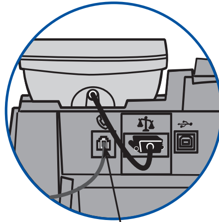
Plug phone line in here
