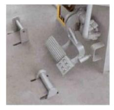
**Brake Pedal**. Single brake pedal simplifies operation by braking tracks on both sides.
