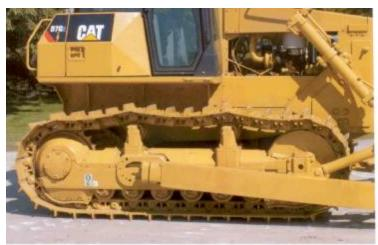
**Roller Frame**. Track roller frames are strengthened box-section structures. Each side is fitted with 6 life-time lubricated track rollers, and there are top rollers mounted on the outside, two on each side.
