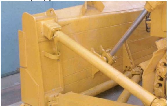
**Dozer Blades**. All dozer blades have a solid, box-section design to prevent twisting and deformation. Dozer blades are made from Caterpillar DH-2<sup>TM</sup> steel, which has extremely high tensile strength and can cope with the toughest work conditions. A heavy-load scraper board structure, hardened mounting bolts, and blades and edge blades increase strength and durability.
