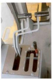
Steering Control Device. The device for steering and operating the gearbox is located to the left of the operator. Operation is comfortable and easy.
