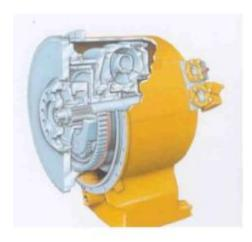
Torque Divider. The torque divider configuration is exclusively Caterpillar's. During lower engine loads, for example when backfilling ditches or spreading materials, it not only has direct-drive efficiency, but also is able to achieve large torque multiplication for loads.
