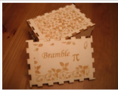
Both bottom and top of the case are laser engraved.
