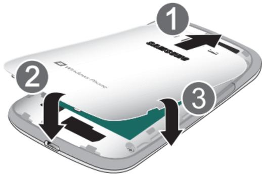
5. Press down firmly along the edges of the cover to ensure that the cover is flush with the phone (4). You should hear a light click as the cover locks in place.
