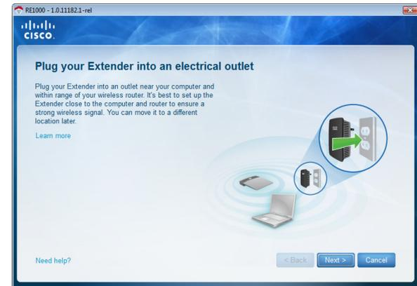
3. Connect your extender to an AC power outlet. Your extender searches for wireless networks. The list of networks is displayed.
