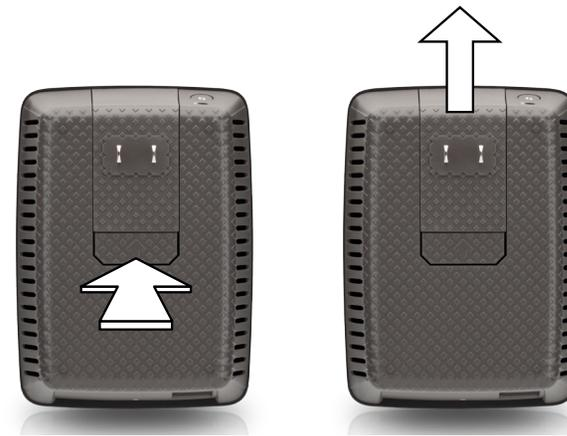
2. Slide the clip cover into the slot that held the AC plug, then connect the AC cable to the power connector.
