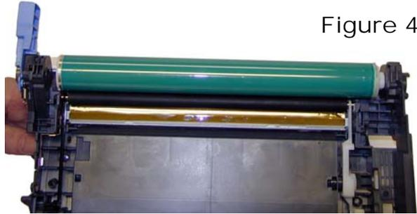
22) Slide the drum axle in from the contact side. Make sure you do not damage the copper drum contacts. Both tabs must be in contact with the axle. See **Figure 45**
