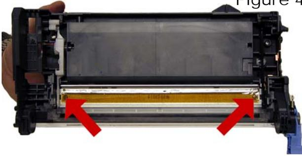
19) Clean off the old conductive grease from the PCR ends, and clean the PCR. Coat both ends of the PCR with a small amount of new conductive grease. Place the plastic stabilizers on the shaft, and install the assembly in the cartridge. See **Figures 41 & 42**
