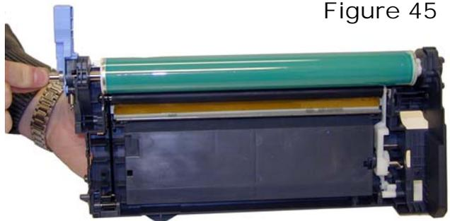
23) Align the drum hub and axle so that the holes line up. Insert the larger of the two metal pins and tap into place with the pin punch. Make sure the pin is centered on the axle. See **Figure 46**
