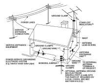
NOTE TO CATV SYSTEM INSTALLER: This reminder is provided to call the CATV system installers attention to Article 820-40 of the National Electrical Code that provides guidelines for proper grounding and, in particular, specifies that the ground cable ground shall be connected to the grounding system of the building, as close to the point of cable entry as practical.
