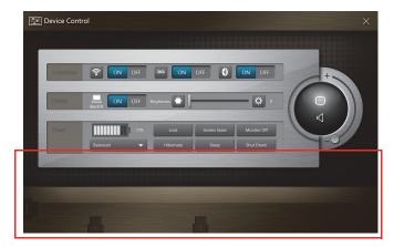
If you have any devices plugged into a USB port or the HDMI port, Device Control will show what type of device is plugged into each port. If you have inserted a storage device into a USB port, you may tap the USB icon to open a context menu. Tap **Open** to view the files in Windows Explorer.
