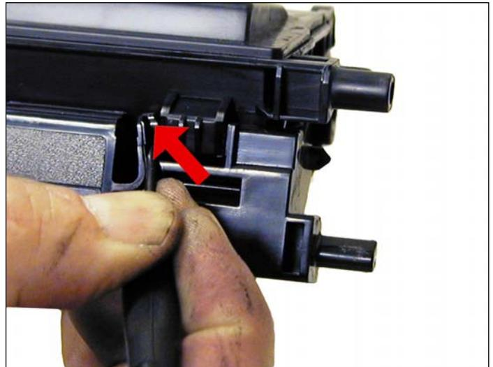
3. Remove the handle by sliding the handle to the right and pulling back on the tab with your finger.
