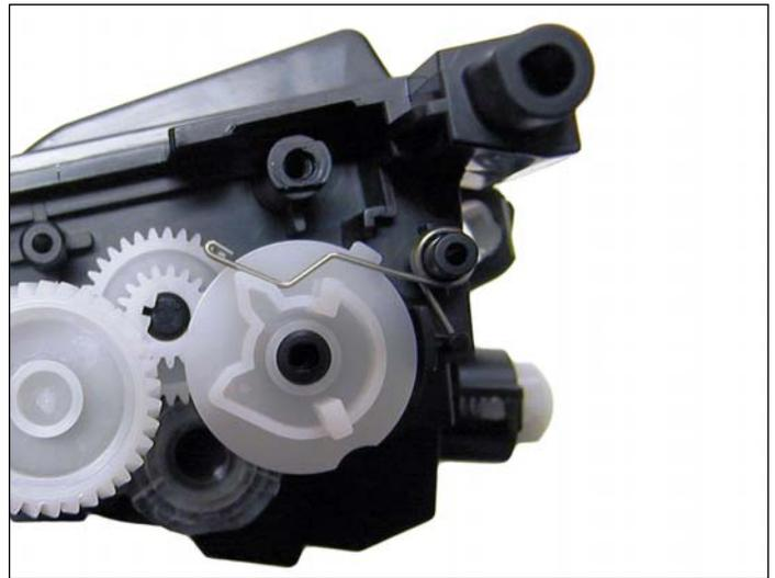
19. Set the reset gear and spring as shown. The tail of the spring fits into a notch at the base of the gear. There are different gears for the TN-110 and TN-115. Each should be set as shown.
