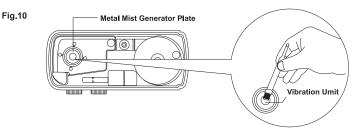
NOTE: How often you should perform this special maintenance depends upon the hardness of the water you are using and how quickly mineral deposits form on the interior surfaces of the humidifier.
