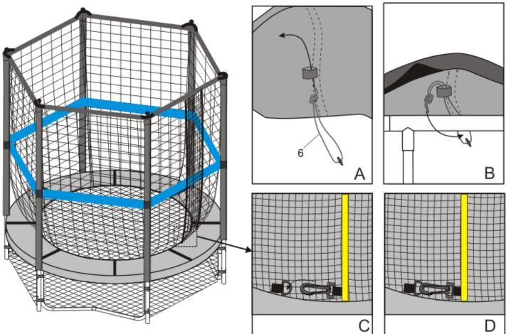
Tie the Elastic buckle (6) located at the under side of the frame pad to the frame.
