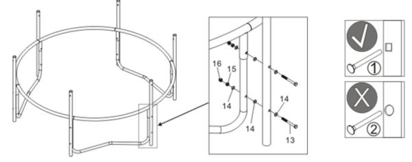
Attach Steel Pipe A (7), to the trampoline frame using the included wrench as shown in the diagram above.
