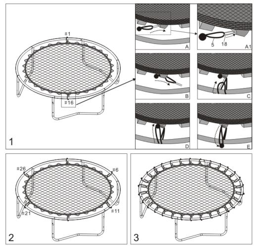
Insert a Ball and Elastic buckle (5) through each fabric loop on the trampoline mat. If needed, use the Steel Wire (18) as shown in Figure A to pull the buckle through the fabric loops on the trampoline mat. Make sure to rotate the ball end of each buckle down to the underside of the mat (see Figure E). Repeat for the other Ball and Elastic buckles. **Be careful of pinch points during assembly**
