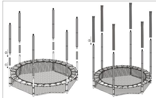
Connect the assembled poles (Steel Pipes B and C) to Steel Pipes A (7). Once attached, place the Pole Covers (10) onto the fully assembled enclosure poles.
