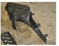
Then remove the two screw on the side of the oil cooler covering that have a large flat washer on them. Use the size 27 torex for this one.
