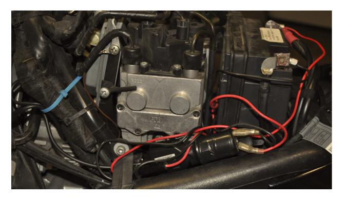
This is how I ran the wires. I used the blue cable ties (They should be black to be politically correct.) to secure the extra length of wires.
