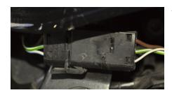
To help in disconnecting the electrical connector (for the fuel pump) you can lift the rear of the fuel tank up to allow you to more fully grip the connector to pull it apart. You have to squeeze the two tabs and pull left.
