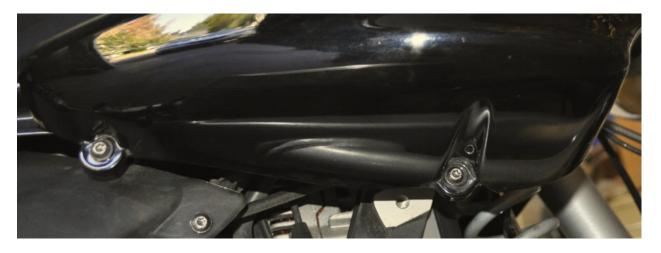
Remove these two screws using the size 25 torex. Then gently remove the plastic cover by prying it up from its mounts on the top. (See oil cooler picture below) Once removed the oil cooler is shown here:
