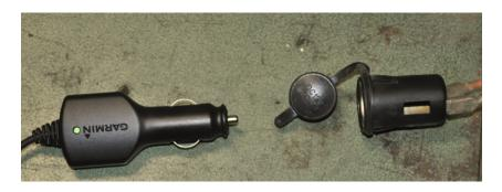
Finally, push the Garmin power cable into the female power coupler and then wrap some electrical tape around the two units to prevent water from entering the connectors. This connector sits under the gas tank, but the front of the gas tank is open to the weather and moisture will get in if you are riding in rain.
