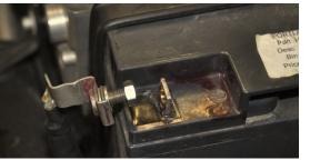
the ground (-) side of a battery first to avoid arcing to ground from anything hot.
