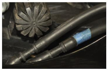
Two prevent misconnecting the lines when you get ready to install the fuel tank I placed a colored tape on one of the lines. The connectors simply pull apart, so do so carefully.
