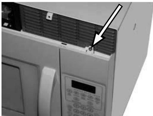
5. Push the panel up to release the tabs from the slots. Pull the panel away from the microwave unit to gain access to the back side of it.
