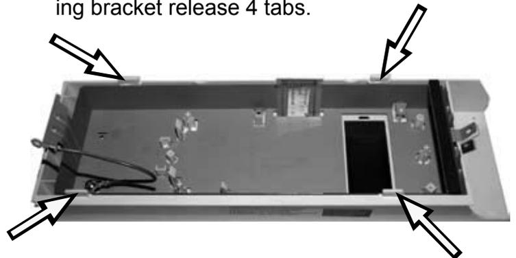
f) Pull the bracket out of the touch panel assembly.
