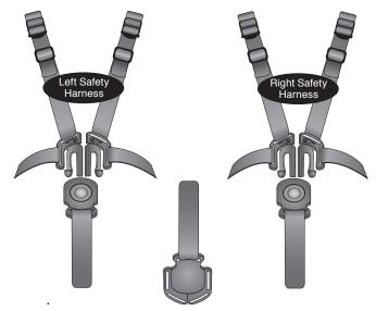
2. Snap the left shoulder strap from the right set of safety harnesses into the center lap buckle. Then, snap the right shoulder strap from the left set of safety harness into the center buckle.
