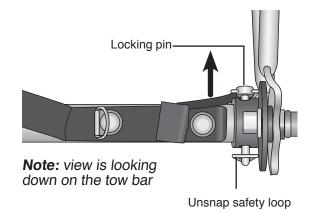
**4.** Remove the tow bar from the tow bar coupler plate.
