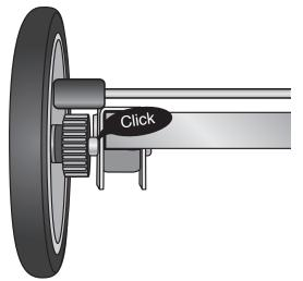
**3.** Pull firmly on the wheel to ensure the locking mechanism is engaged. Repeat these steps on the opposite side.
