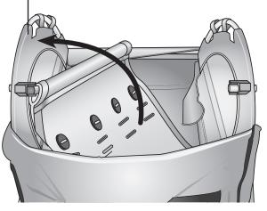
**3.** Rotate the crossbar into the joiner housing.
