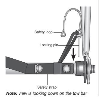
7. Slide the metal safety loop onto the locking pin. Check that it is securely in place.
