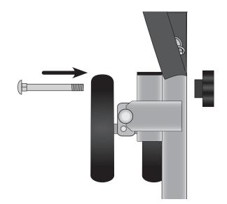
**4** Tighten the knob so the front wheel attachment is securely attached to the tow bar.
