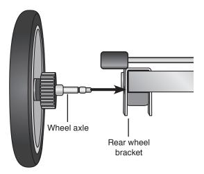
**2.** Push the wheel into the bracket until you hear the axle click into place.
