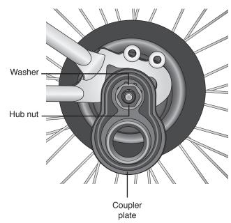
**5.** Insert the tow bar into the large hole on the coupler plate.
