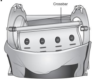
**4** Depress outside buttons on crossbar to insert in joiner and lock into place.
