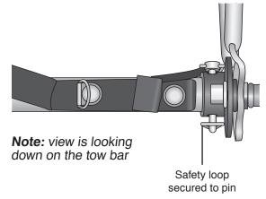
8. Wrap the tow bar safety strap around the bicycle frame and clip it to the ring on the end of the tow bar.
