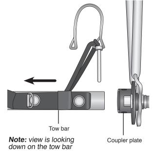
**5.** Re-insert the locking pin into the holes on the end of the tow bar. Snap the safety loop onto the locking pin.
