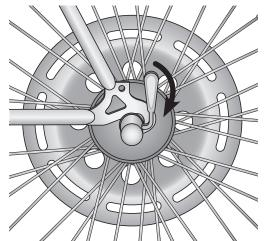
**2.** Remove the axle skewer and spring. Leave the wheel in place.
