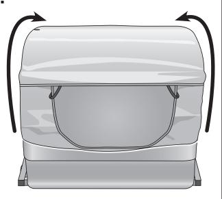
2. Snap the canopy in place, there are 2 snaps on each side, then secure with the hook and loop fasteners.
