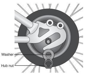
**2.** Place the tab washer on the axle. Fit the tab into the slot on the bicycle frame dropout.
