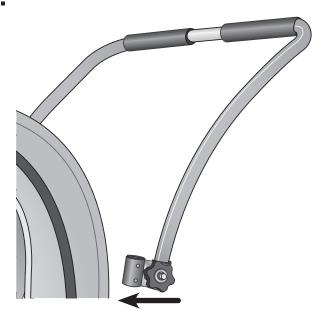
**2.** Turn the attachment knobs (both sides) until they are firmly in place.
