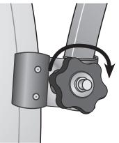
**3.** Check the handlebar by pulling back and forth to ensure it is securely attached to the frame.
