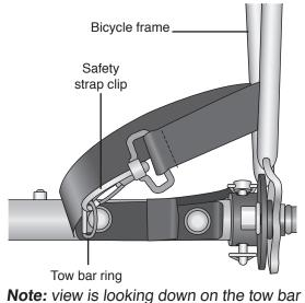
**3.** Unsnap the safety loop and remove the locking pin from the tow bar coupler plate and tow bar.
