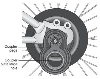
4. Place the hub nut and washer back on the axle and tighten.
