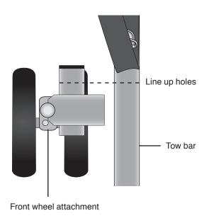
**3.** Attach the front wheel attachment to the tow bar and insert the bolt.
