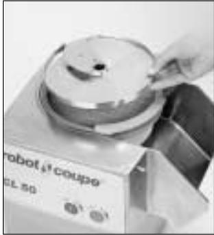
Rotate the plate until the slot in the plate hub falls over the motor shaft pin. Continue to rotate one full turn. If the cutting plate scrubs the grid-do **not proceed**. Call your **authorized service agency**.
