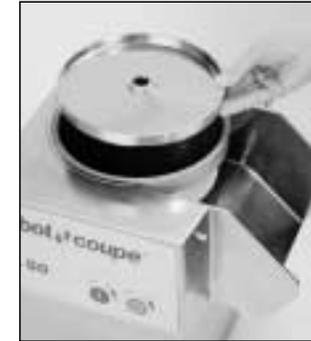
motor shaft. Continue to rotate the blade a full 360 degrees to make sure the plate doesn't scrub against the plastic grid. **If rubbing occurs-do not proceed. Call your authorized service agency.**
