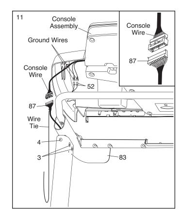
Set the console assembly on the Left and Right Handrails (82, 83). Be careful not to pinch any wires. Insert the excess Upright Wire (87) into the Right Handrail.
