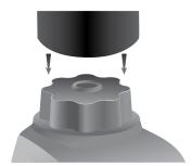
**NOTE:** When properly positioned, pitcher or accessory jar assembly will rest completely on Blender base. If not, repeat steps 3 and 4.
