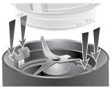
4. Press down and rotate pitcher or accessory jar clockwise, approximately 1/4 turn through two steps of resistance.
