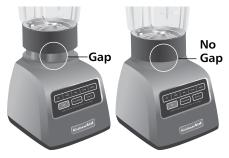
**NOTE:** If a gap exists between the locking collar and the base, the pitcher or accessory jar might not be locked into the locking collar or the assembly is not positioned properly on the Blender base. See Blender Assembly, page 8 for further instructions.
