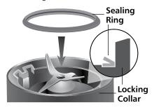
**NOTE:** For easier jar and collar assembly, you can dip the gasket in water before placing it into the collar. A damp gasket makes it easier to attach the glass jar to the collar.
