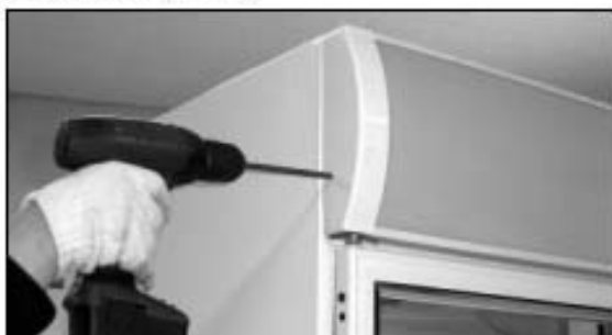
1. Unscrew the left sign frame.
