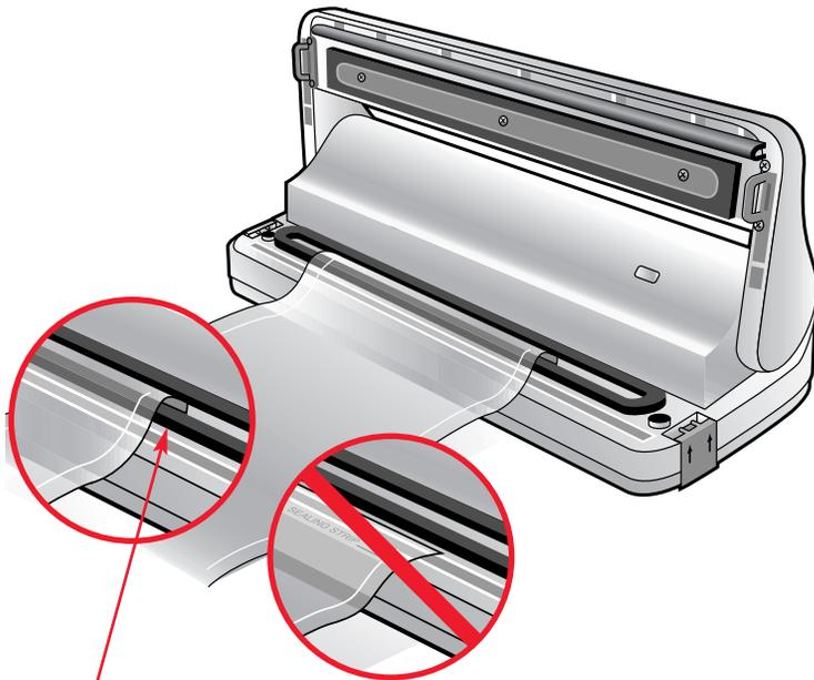
**IMPORTANT:** Make sure the open end of the bag touches the blue label on the bottom of the vacuum channel.
