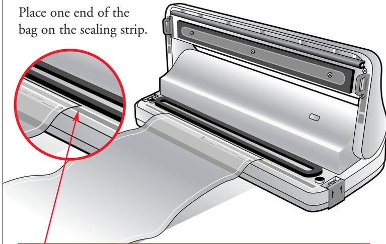
**IMPORTANT:** Make sure the end does not go over the black foam rubber ring, or into the vacuum channel.
