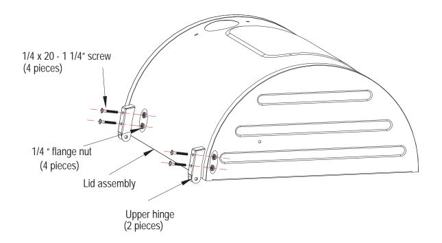
Place lid assembly on top of firebox then align hinge holes. Attach lid to firebox using 2 hinge pins. Once hinge pins are in place, insert hitch pin into hole in hinge pins.
