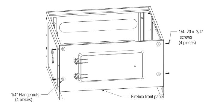
Assemble 2 left legs, 1 right rear leg and 1 right front leg to firebox and bottom shelf. Use four  $1/4-20 \times 2 \frac{1}{2}$  "screws for the bottom shelf and eight  $1/4-20 \times 3/4$ " screws for firebox, tighten screws as shown in the figure.
