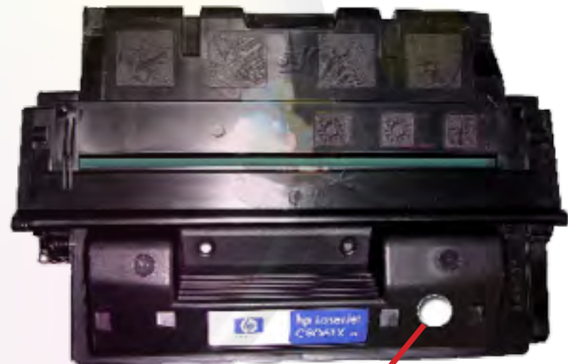
Create Refill Hole Here
