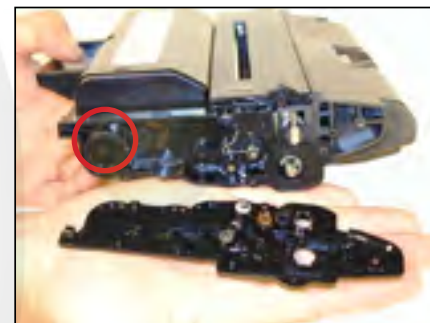
D. Remove plug (circled in red) and remove any remaining toner before refilling.
