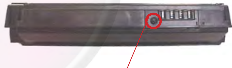
Remove screw to replace chip
