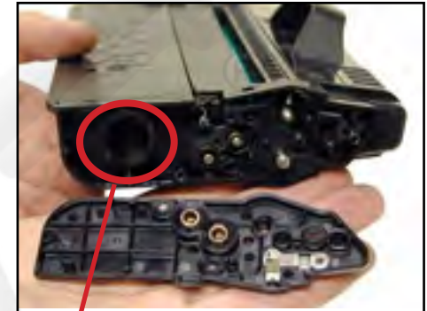
Carefully remove Toner Plug.
