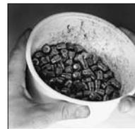
Gently shake the bullets in an orbital motion to coat the bullets. If they do not coat completely, add a little more lube.
