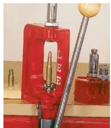
**4** Seat the bullet and crimp it in place. Full length sized ammunition is usually improved with a factory crimp. (See next page)
