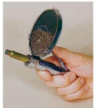
**2** Install a new primer. Picture shows this operation using the Lee Auto-Prime, the most popular priming tool ever made. (See page 24)
