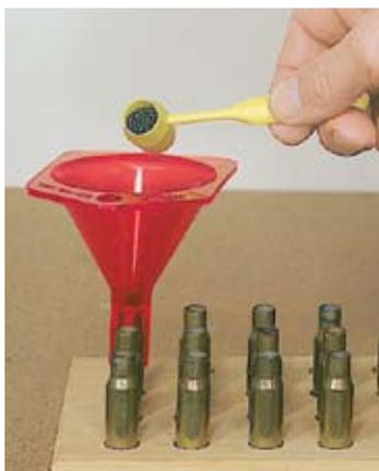
**3** Add a charge of powder. Lee dies, except RGB, include a powder dipper and extensive load data to tell you what kind of powder to use.
