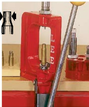
**1** Remove the old primer and size the case. This is usually done with the same die. Cases can be full length sized or only neck sized for best accuracy.
