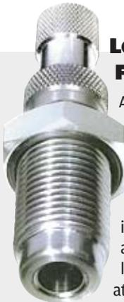
A carbide sizer sizes the cartridge while being crimped so every round will positively chamber freely with factory like dependability. The adjusting screw quickly and easily sets the desired amount of crimp. It is impossible to buckle the case as with a conventional bullet seating die. Trim length is not critical so this extra operation takes less time than it would if cases were trimmed and chamfered.
