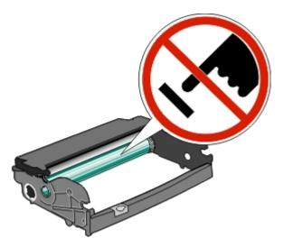
**6** Insert the toner cartridge into the photoconductor kit by aligning the rollers on the toner cartridge with the tracks. Push the toner cartridge until it *clicks* into place.
