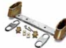
34-306A Bronze Gibraltar double anchor set, jigged for easy install, with wedges and stainless escutcheons, for ring style handrails. Use with RRH-100 and CRH-100.
