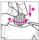
WAIT AT LEAST 3 MINUTES BEFORE REMOVING THE PRESSURE LOCKING SAFETY CAP. This allows the pressure inside the tank to dissipate.
