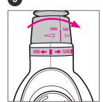
Press accessory attachment onto the Steam Nozzle and rotate to the "Closed" position.
