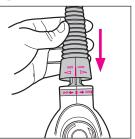
To attach the Concentrator Nozzle, Flexible Extension Hose or Garment/Surface Attachment, line up the indicator line on the accessory attachment with the indicator line on the handheld unit.
