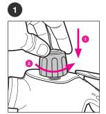
Push down on the Pressure Locking Safety Cap until the cap "clicks". While cap is pressed, turn counterclockwise to remove.
