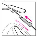
To access continuous steam push the Continuous Steam Lock to the "locked" position.
