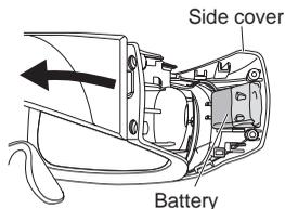
3. Remove the battery from inside the side cover, and cut the two wires one by one with scissors.
