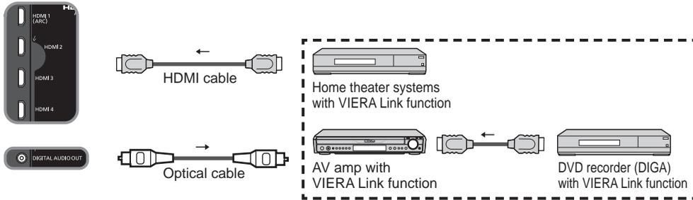
No optical cable is necessary when connecting a Home Theater supporting "HDAVI control 5" with an HDMI cable. Audio will be supported via ARC (Audio Return Channel) (p. 34)
