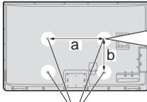
Holes for wall-hanging bracket installation
