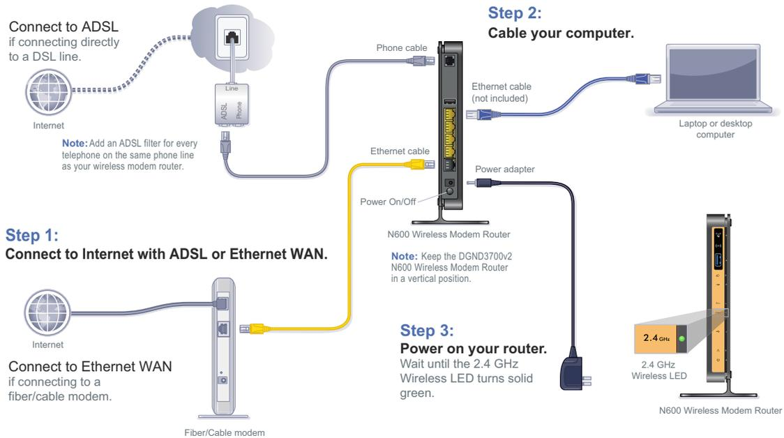
Figure 7. Cabling diagram
