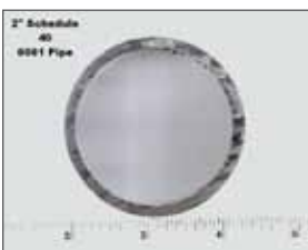
2" schedule 40 aluminum pipe frame 2.375" O.D. - 2.067" I.D.
