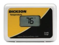
**SP425** Temperature Logger. Digital Display. Accuracy ±1.2°F, ±0.67°C. Range -4 to 158°F, -20 to 70°C.
