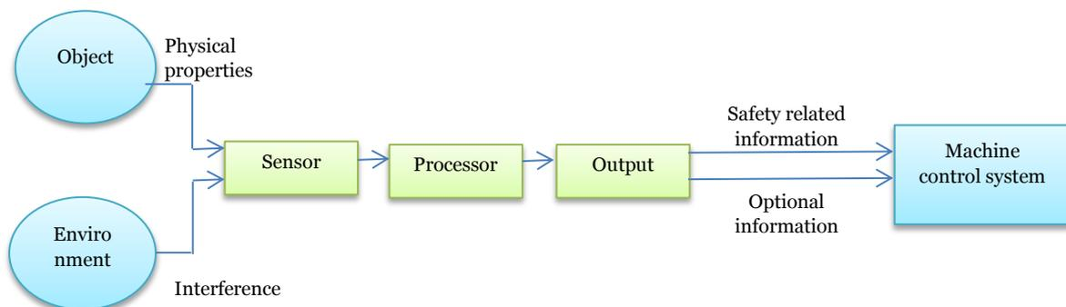
Figure 1. Example of architecture for Safety Related Sensor (SRS)
