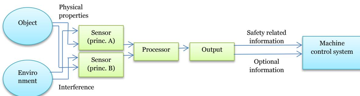
Figure 2. Example of architecture for Safety Related Sensor (SRS) with two sensors
