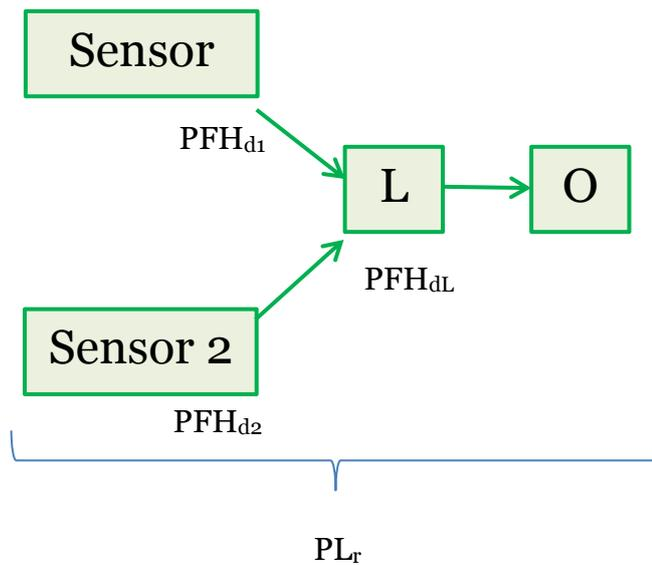
Figure 7. Simplified block diagram for the safety function "detect obstacle and brake"
