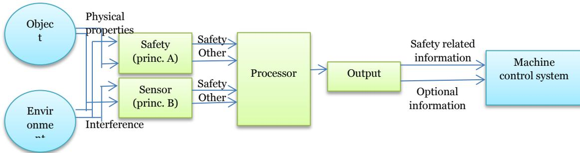
Figure 3. Example of architecture for Safety Related Sensor System (SRSS) with two sensor units
