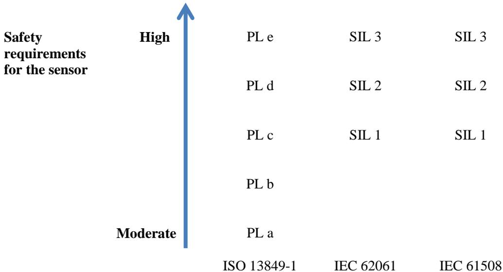
Figure 5. Comparison between safety levels of different standards
