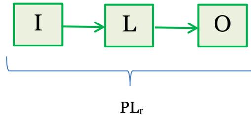
Figure 6. Simplified block diagram for the safety function "detect obstacle and brake"
