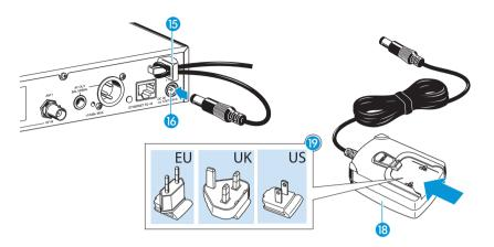
Only use the supplied NT 2-3 mains unit. It is designed for your receiver and ensures safe operation.
